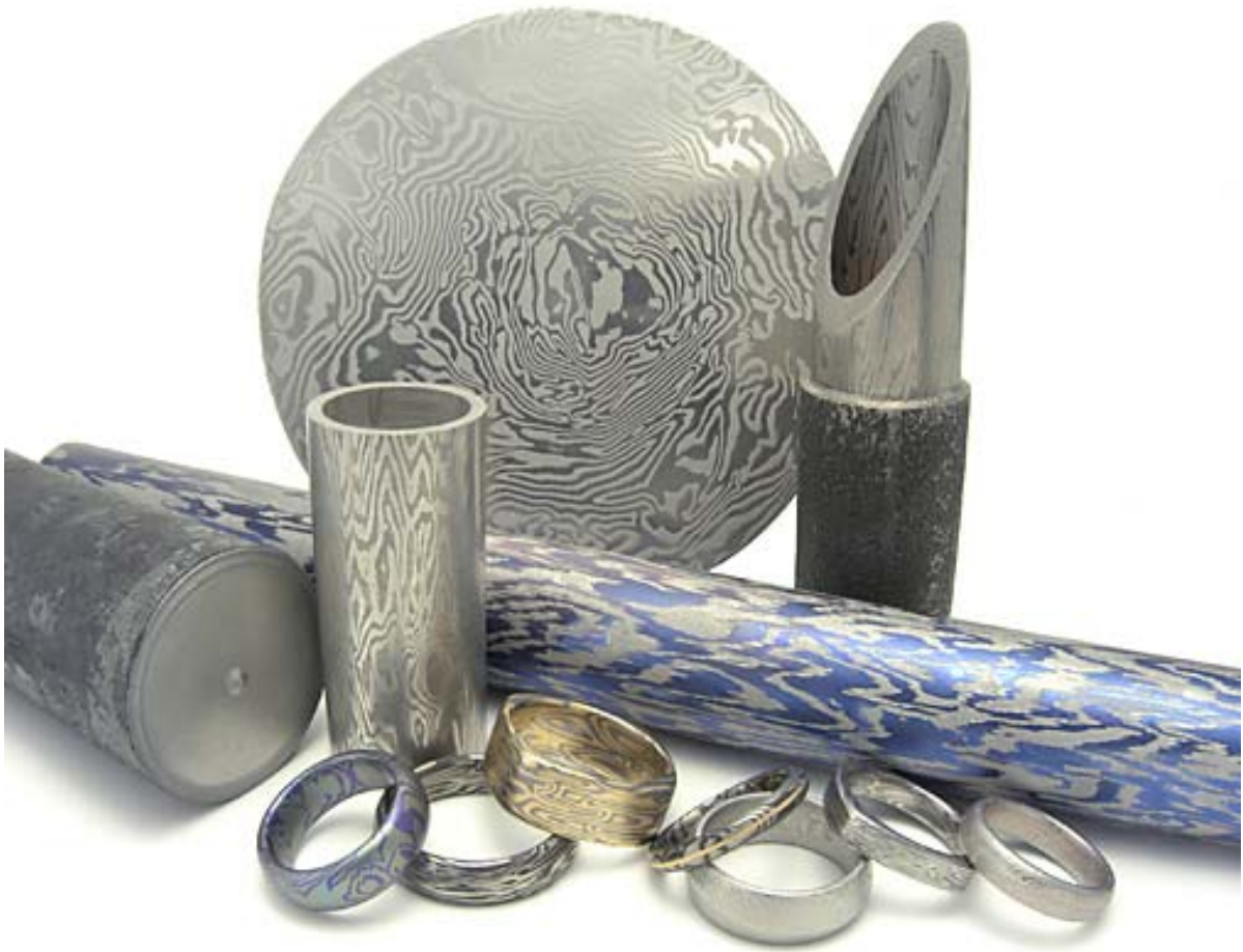
A variety of XPMs utilizing titanium, tantalum, platinum, 18K gold, and stainless steel – 2008.
