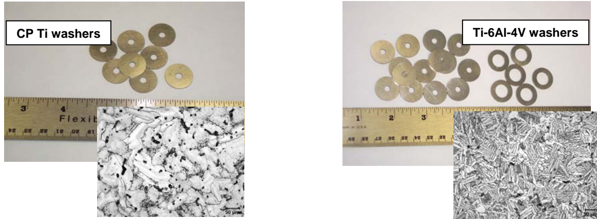
Figure 4: C.P titanium and Ti-6Al-4V washer components produced by die pressing + sintering.
