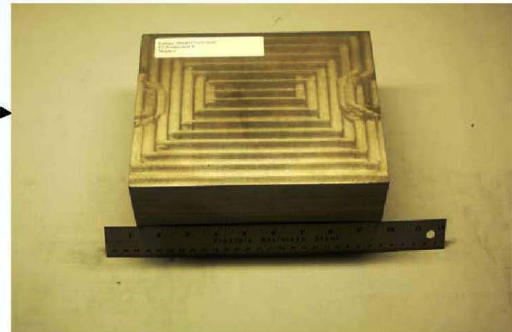
Ti-6Al-4V infiltrated with 90%Mg - 10%Al
