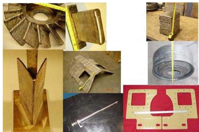
Figure 9: Example Titanium Components Produced by the Rapid Manufacturing Plasma Transferred Arc System
