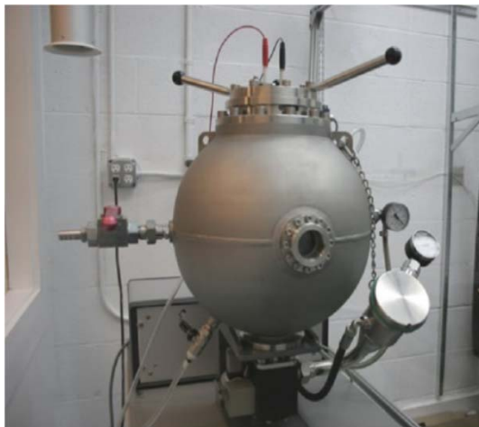
20L test chamber for explosivity testing – ASTM E-1226
