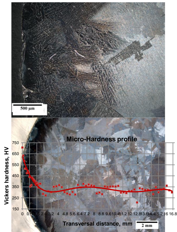
Figure 1. Alpha-case layer after investment casting of Ti6Al4V alloy, and the microhardness profile from the edge into the core of cast.
