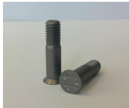
Figure 8: Titanium countersunk rivets treated with the \text{TiO}_2 -nanotube anodizing
