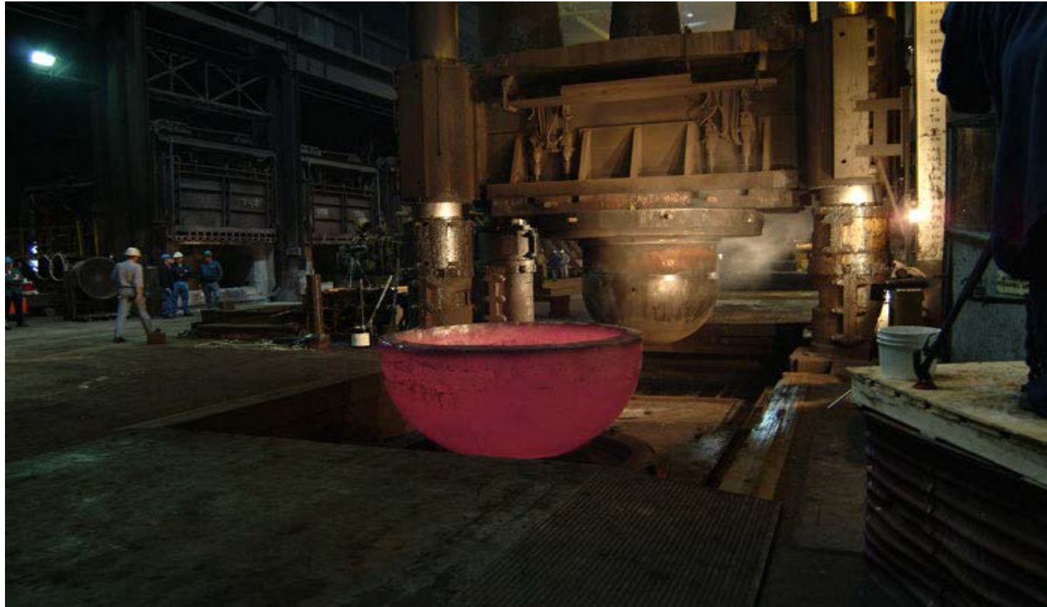
Ladish Forging in Cudahay, WI, heated and shaped 6 Al- 4V ELI titanium ingots into discs which were then formed into hemispheres (Photo courtesy of Woods Hole Institution)
