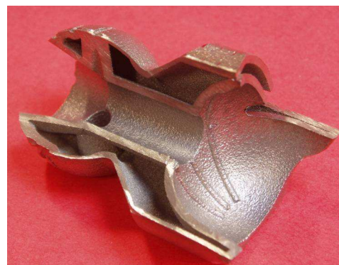
Figure 2. Ti64 part. One section removed to reveal internal structure. Courtesy of HIPP medical AG.
