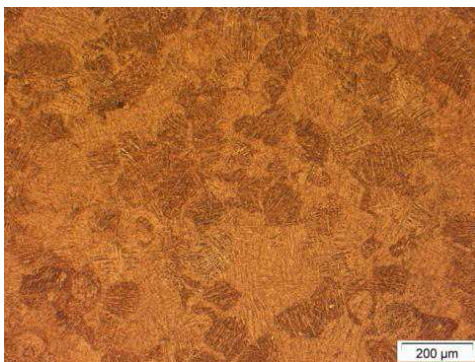
Figure 10. EOS Ti64 after 1h in 800°C. Etchant Kroll's reagent.
