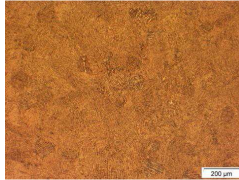
Figure 11. EOS Ti64 after 1h in 850°C. Etchant Kroll's reagent.
