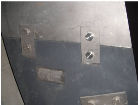
Pueblo Viejo AUT-150: Compartment 1 head baffle clamping connection between lower two (2) pieces.
