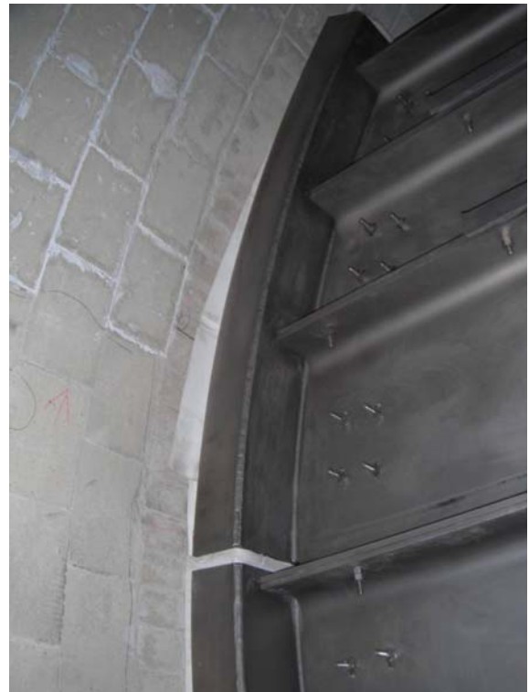
Pueblo Viejo AUT-150: Reverse (discharge) side of compartment 1 wall. Stiffener rings, clamping plate and titanium hardware.
