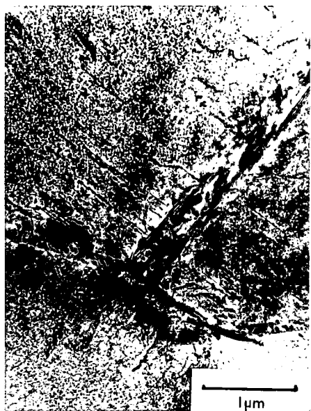
d) The precipitate dispersion in Ti5%Zr1%Si aged to peak hardness at 550°C.
