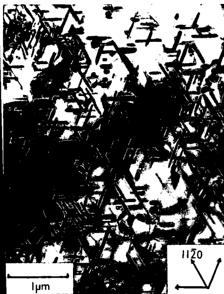
c) The precipitate dispersion in Ti1%Si aged to peak hardness at 550°C.
