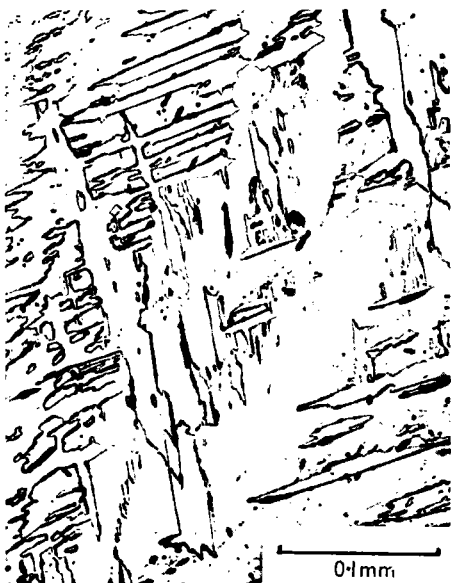
a) Light micrograph of Ti1%Si after water quenching from 1200°C.
