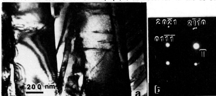
Figure 2. Starting microstructure following the first heat treatment cycle (a) wrought material annealed at 1035°C for 15 min/WQ (b) RS material in the as-solidified condition.
