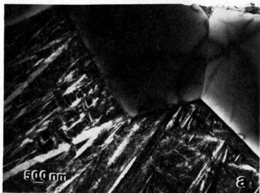
Figure 9. TEM micrograph of RS alloy showing hexagonal close-packed equiaxed grains (a) \alpha , after annealing at 925^\circ\text{C}/24 hr; (b) SAD of [01\bar{1}2] \alpha -Ti zone in equiaxed grain.
