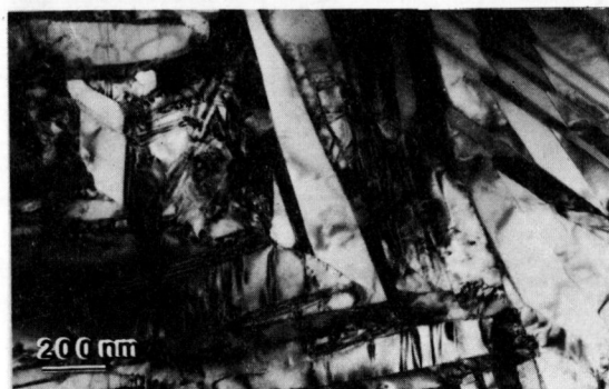
Fig. 4. TEM micrograph of as-quenched RS specimen. This microstructure displays short martensite plates with microtwins.
