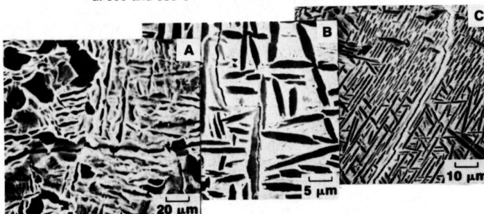
Figure 11. Fatigue Crack Propagation Through Ti-6246 LCF Specimens. A-alpha-beta Processed (Forging-4I), B,C - Beta Processed (Forging-5I)
