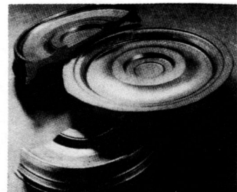
Fig.3. Isothermally Forged Compressor Discs
