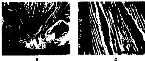
Figure 10. SEM fractograph of crystallographic crack initiation typical of both conditions A and B. This specimen was tested at 1.0% total strain range for condition B. (a) crack initiation and (b) propagation on crystallographic faces is by shear along the finer alpha platelets.
