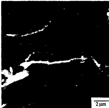
Figure 7 - Cleavage crack nucleated in a primary \alpha_2 particle in microstructure 4.
