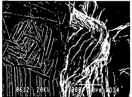
Fig.(6.c) Crack growth along the \alpha /B interfaces. T16246, 480°C.
