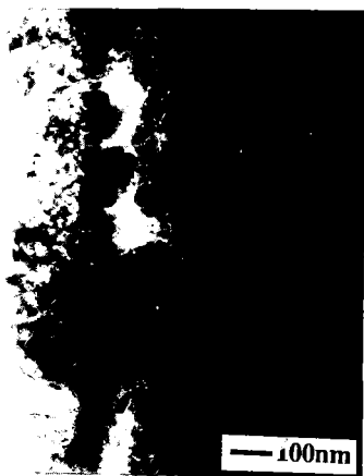
Figure 7. TEM micrograph of cross-section oxide on IMI834 after 100h at 600°C.
