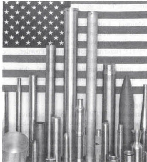
Figure 8. Flowforming produces extremely straight and concentric parts 40 .
