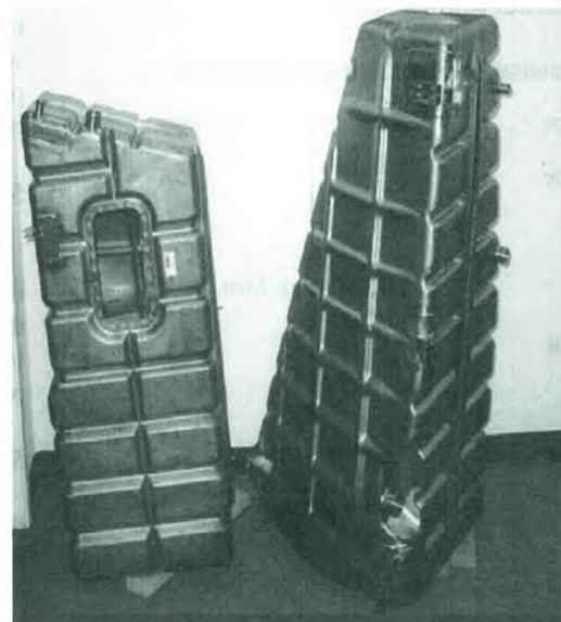
Figure 5. Ti-6Al-4V fresh water tank for Boeing Business Jet/737, deep integral ribs for stiffening 34 .
