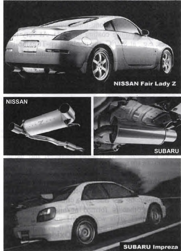
Figure 5. Application examples of titanium exhaust systems in Japanese passenger cars (courtesy of Toshihiko Saiki)
