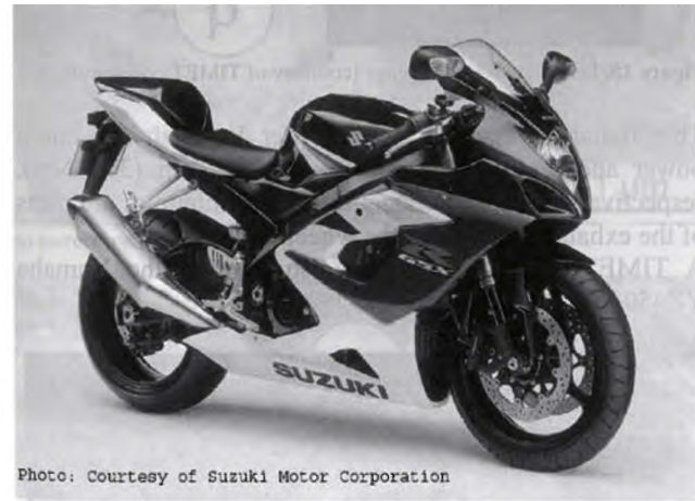
Figure 14. Suzuki GSX-R1000 featuring a Ti-1.5Al exhaust system
