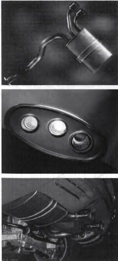
Figure 4. Exhaust system of the Corvette Z06 (courtesy of TIMET company)
