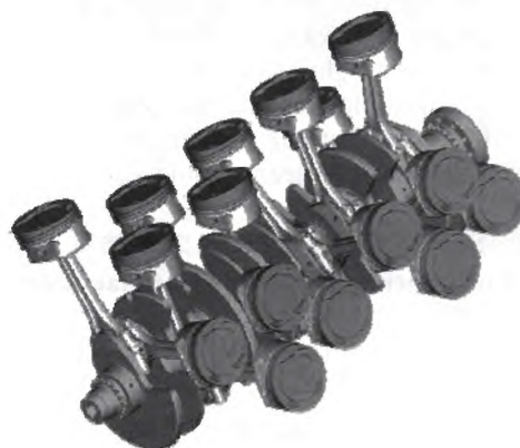
Figure 2. 16 Ti-6Al-4V connecting rods in the Bugatti Veyron's engine
