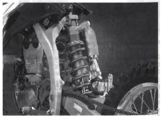
Figure 19. TIMETAL LCB suspension spring of the Yamaha YZ450F (courtesy of TIMET company)
