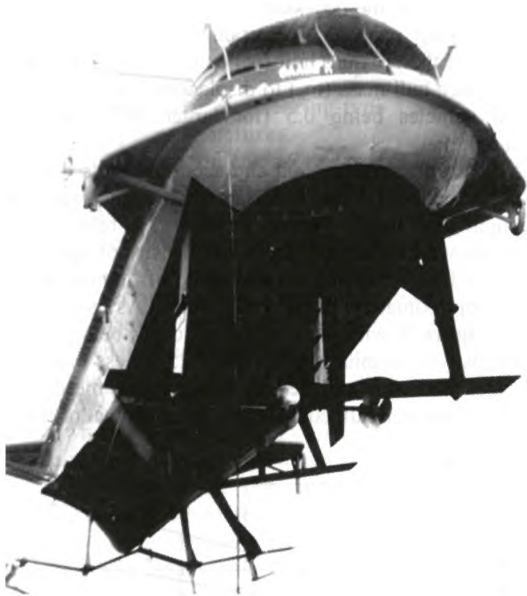
Figure 8. Fore and aft titanium hydrofoil arrangements of "Kometa"-type vessel, Greece.
