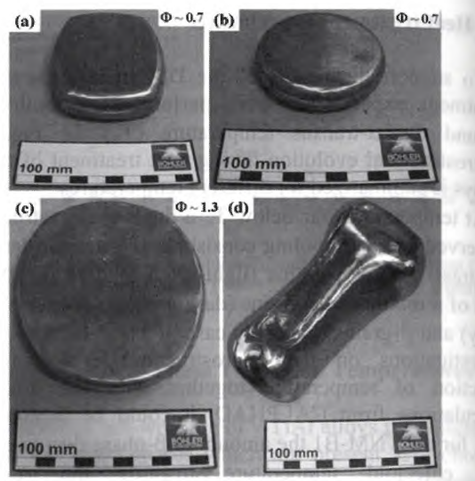
Figure 7. TNM-B1 billets after side-pressing to an overall strain of 0.7 (a), upsetting to an overall strain of 0.7 (b), and side-pressing to an overall strain of 1.3 (c). (d) Grinded TNM-B1 blade pre-form manufactured by upsetting both sides of a cylindrical bar and consequent side pressing to the final shape.
