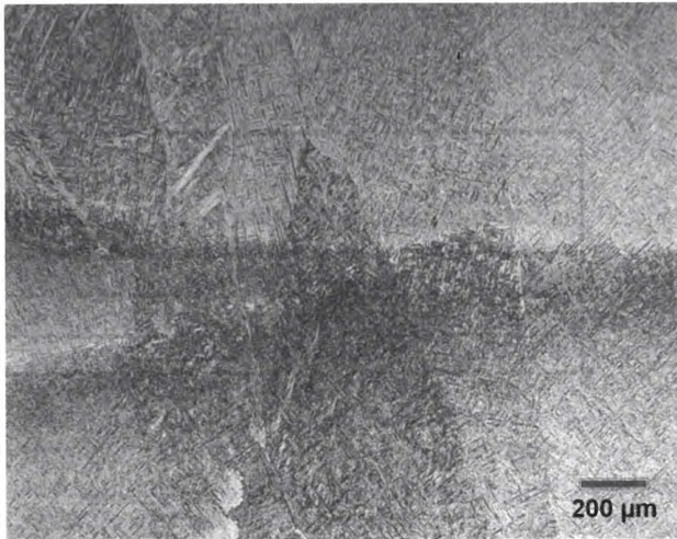
Figure 8A. Microstructure of weld metal, center area of XH6005-B Plate
