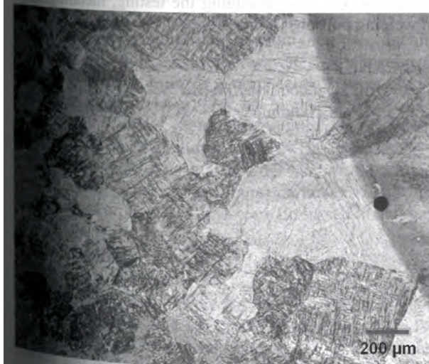
Figure 7A. HAZ of welded plate
