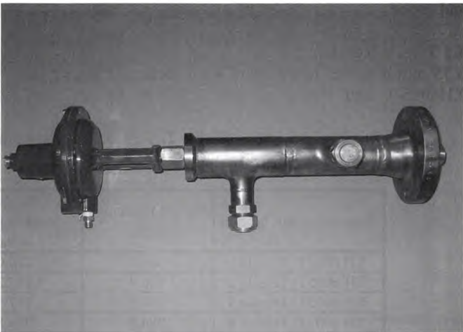
Figure 2. Reaction apparatus for the Armstrong process
