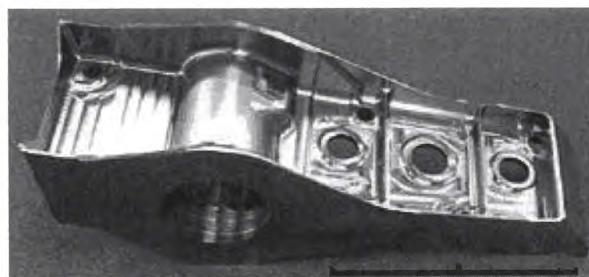
Figure 3. Fully machined LAM F-15 Pylon Rib (Courtesy DoD ManTech)
