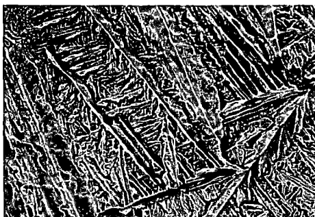
Figure 8 : cumulative annealings, \beta \rightarrow \alpha transition
