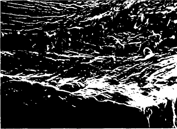
Fig. 7 : (SEM). "Cleavage type" fracture propagating on various parallel planes. \Delta K = 29.1 \text{ MPa}\sqrt{\text{m}} . Magnification 800 times.
