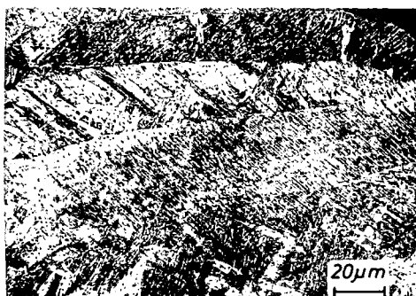
Fig. 7 Large \beta -grains in the microstructure of bead on plate welded titanium ( J = 220 A, U = 36 V, v = 35 cm/min, flux \text{CaF}_2 + \text{SrCl}_2 )
