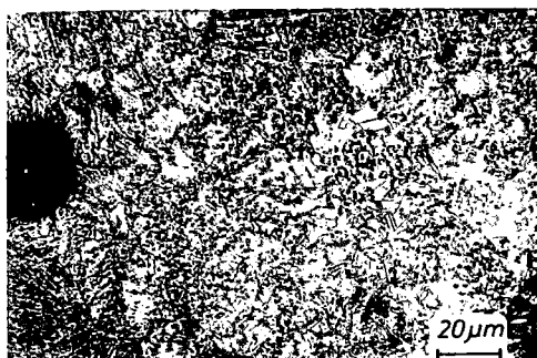
Fig. 5 Pore in the microstructure of bead on plate welded titanium ( J = 220 A, U = 32 V, v = 50 cm/min, flux \text{CaF}_2 + \text{K}_2\text{TiF}_6 + \text{SrCl}_2 )
