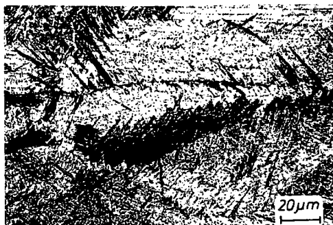
Fig. 6 Crack in the microstructure of bead on plate welded titanium ( J = 220 A, U = 32 V, v = 50 cm/min, flux \text{CaF}_2 + \text{K}_2\text{TiF}_6 + \text{SrCl}_2 )
