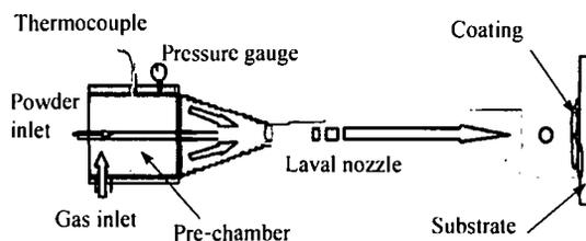
Figure 1. Schematic diagram of cold spray
