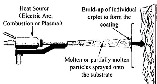
Figure 2. Schematic diagram of coating formation process during thermal spray
