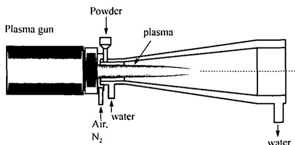
Figure 3. Schematic of a plasma torch equipped with a shroud
