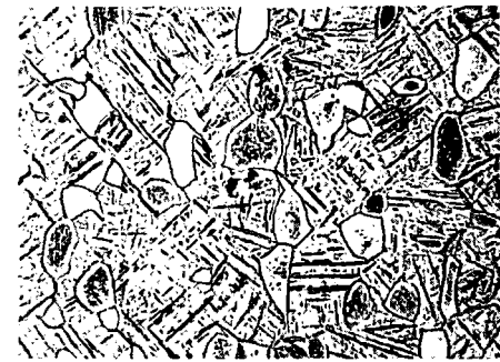
FIGURE 47. MICROSTRUCTURE OF A Ti-6Al-4V ALLOY BOLT HEADED AT 1500 F, AND SUBSEQUENTLY SOLUTION TREATED FOR 1/2 HOUR AT 1700 F AND QUENCHED 1/2HF-1-1/2HCl-2-1/2HNO 3 etch (North American Aviation, Downey, California)
