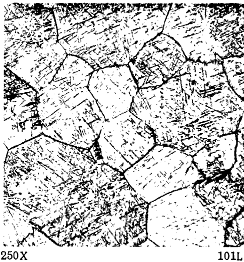
b. Ti-3Al-5Cr (low carbon) as extruded at 1750 F (25HF-25HNO 3 -50 glycerine)
