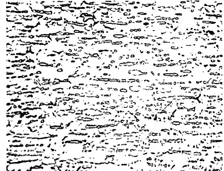
FIGURE 47. MICROSTRUCTURE OF A Ti-6Al-4V ALLOY BOLT HEADED AT 1500 F, AND SUBSEQUENTLY SOLUTION TREATED FOR 1/2 HOUR AT 1700 F AND QUENCHED 1/2HF-1-1/2HCl-2-1/2HNO 3 etch (North American Aviation, Downey, California)
