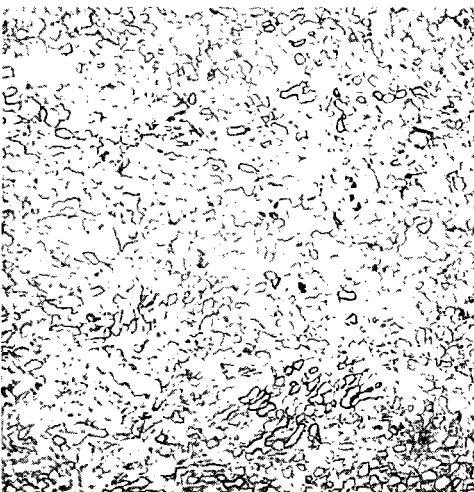
c. Forged, annealed as in b and heat treated 1 hour at 1700 F, quenched, and aged 3 hours at 1000 F
