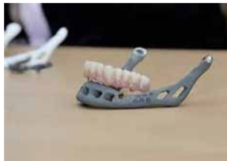
Figure 20c. A Titanium Jaw fabricated by Additive Manufacturing.
