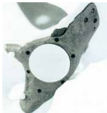
Figure 20b. An Artificial Hip Replacement fabricated using Additive Manufacturing and Electron Beam Melting.
