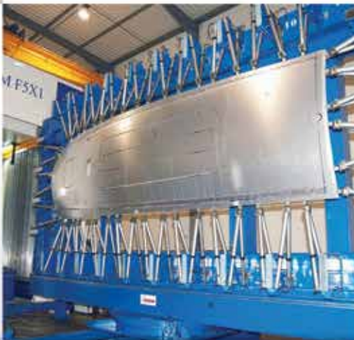
Panel mechanical pocket milling, drilling and trimming
