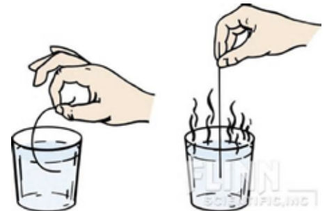
Figure 15. Mechanism of Shape Memory. Nitinol undergoes deformation at one temperature, then recover its original, undeformed shape upon heating above its “transformation temperature.”
