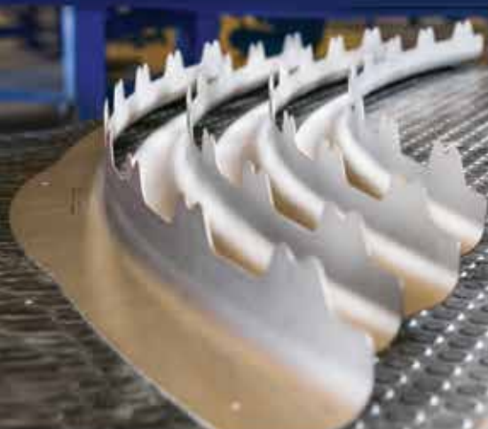
Superplastic Forming and Hot Forming for titanium airplane structural and engine components
