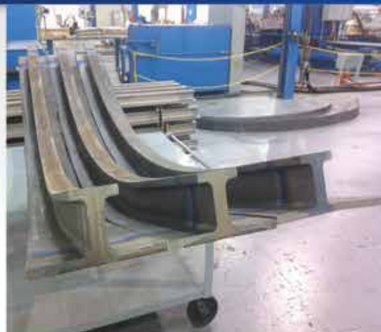
Superplastic Forming and Hot Forming for titanium airplane structural and engine components
