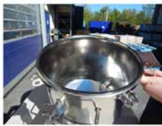
pharmaceutical production vessel electropolished
