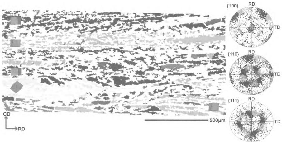
**Figure 5.** Orientation map of the reconstructed  $\beta$  microtexture with the corresponding discrete PFs.
