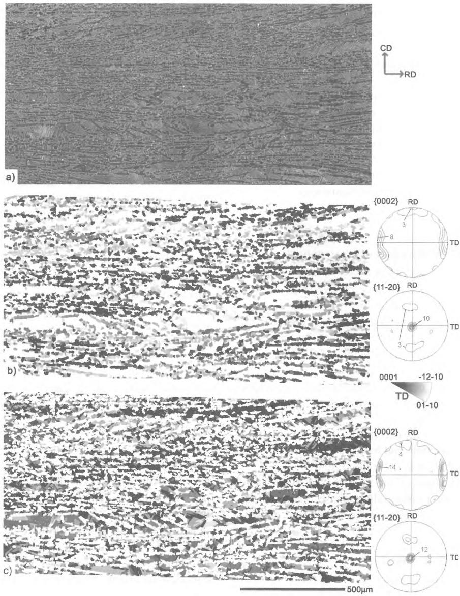
**Figure 4.** a) Microstructure of the analysed region. Orientation maps and corresponding pole figures b)  $\alpha_p$  grains and c)  $\alpha_s$  colonies.
