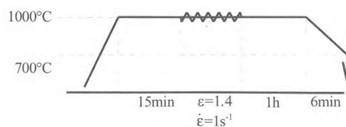
**Figure 1.** Thermo-mechanical processing route
