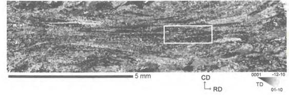
**Figure 3.** EBSD map of the compressed and annealed sample.
