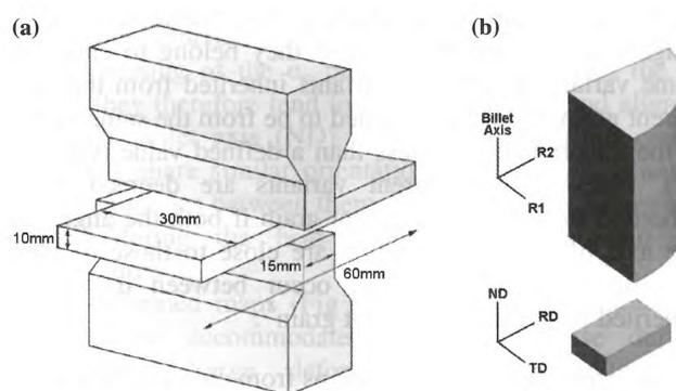
**Figure 1.** (a) Schematic diagram of the plane strain compression test, (b) Orientation of the PSC specimens with respect to the billet.
