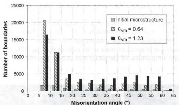
**Figure 6.** Misorientation angle distribution in the reconstructed  $\beta$  phase for the maps in Fig. 5. Note: no data is given for misorientations  $< 5^\circ$ .
