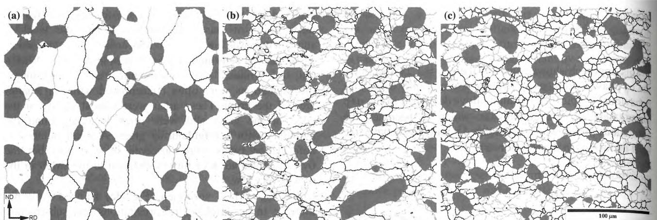
**Figure 5.** EBSD Maps of the reconstructed  $\beta$  phase (coloured white), showing low and high angle grain boundaries. Light grey boundaries  $> 5^\circ$  and black boundaries  $> 15^\circ$ . (a) initial microstructure, (b)  $\epsilon_{vm} = 0.64$ , (c)  $\epsilon_{vm} = 1.23$ .
