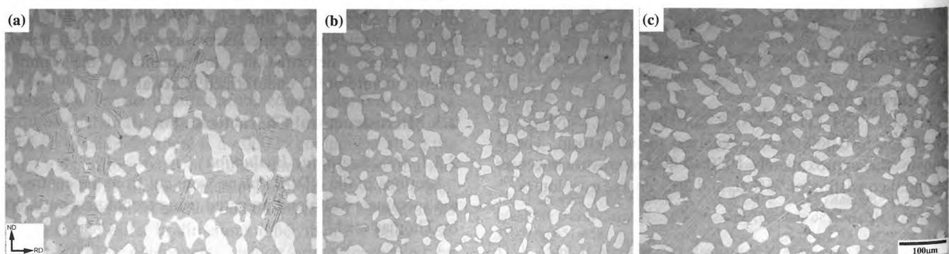
**Figure 2.** Optical microstructures of the PSC specimens: (a) initial microstructure, (b)  $\epsilon_{vm} = 0.64$ , (c)  $\epsilon_{vm} = 1.23$ .
