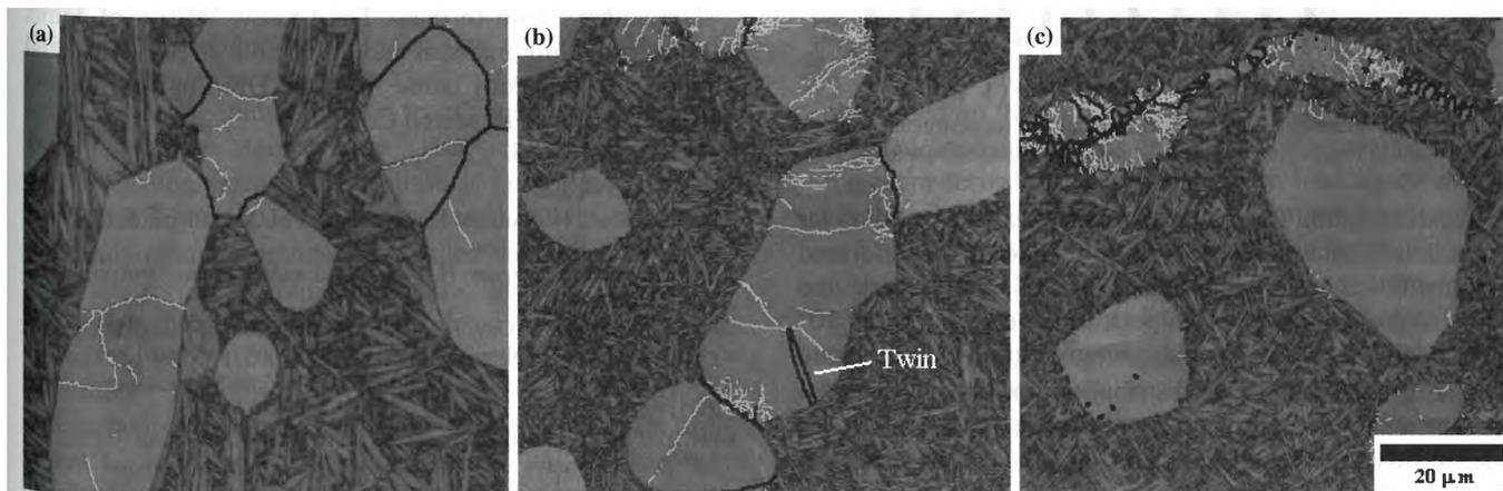
**Figure 4.** EBSD band contrast maps showing low and high angle grain boundaries in the  $\alpha_p$  phase. Light grey boundaries  $> 2^\circ$  and black boundaries  $> 15^\circ$ . (a) initial microstructure, (b)  $\epsilon_{vm} = 0.64$ , (c)  $\epsilon_{vm} = 1.23$ .
