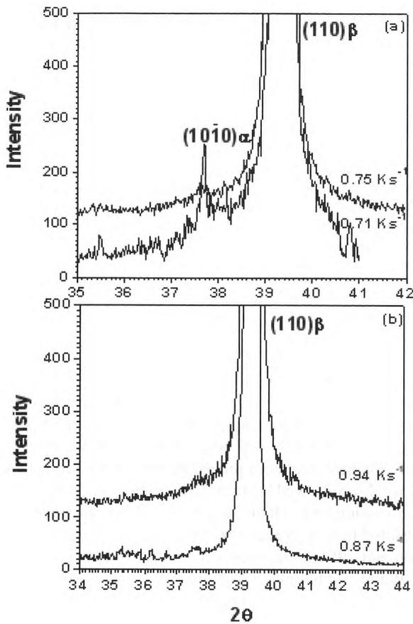
**Figure 1.** Wide-angle x-ray diffraction results for Ti-38644 having grain size of 160 and 295 $\mu\text{m}$  cooled at indicated rates.
