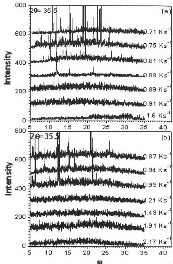
**Figure 2.** Rocking curve x-ray diffraction results for Ti-38644 having grain size of 160 and 295  $\mu\text{m}$  cooled at indicated rates.
