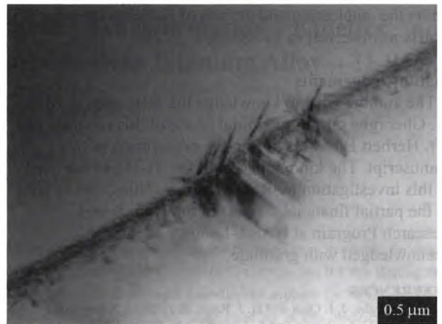
**Figure 5.** Transmission electron micrograph of Ti-3Al-8V-6Cr-4Zr-4Mo showing the side-branching of  $\alpha$  into neighboring prior  $\beta$  matrix following solution treatment at 1228K for 4 h and quenched at  $0.71\text{Ks}^{-1}$ .
