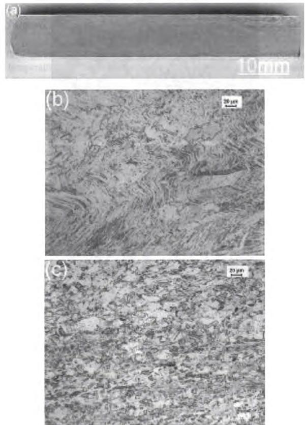
**Figure 3.** (a) Macrostructure of a Ti-46.3Al-2.5V-1.0Cr-0.3Ni pancake forged to 85% height reduction, and the microstructures in the stagnant zones of (b)Ti-46.3Al-2.5V-1.0Cr-0.3Ni and (c)Ti-46.3Al-2.5V-1.0Cr-0.3Ni-0.15Gd, respectively.
