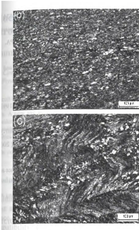
**Figure 2.** (a) Typical macrostructure after forging to a height reduction of 70% in Ti-46.3Al-2.5V-1.0Cr-0.3Ni, showing the stagnant zone near the top and bottom surfaces, the insufficiently recrystallized zone at the free side surface and the uniform flow zone in the middle; (b) microstructure in the uniform flow zone showing well recrystallized and spheroidized grains, and (c) microstructure in the stagnant zone showing remaining lamellae which were bent due to severe deformation.
