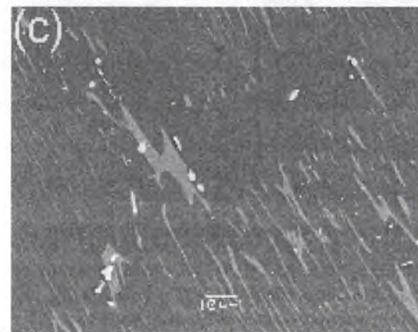
**Figure 1.** (a) Macrostructure and (b) microstructure of the transverse section in the as-cast Ti-46.3Al-2.5V-1.0Cr-0.3Ni ingot; and (c) back-scattered electron microstructure in the as-cast Ti-46.3Al-2.5V-1.0Cr-0.3Ni-0.15Gd ingot. Note the small white Gd-containing particles identified as either Gd oxide or Gd-Al intermetallic in (c).
