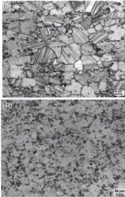
**Figure 4.** Near fully lamellar microstructures after heat treatment of the 85% forged (a) Ti-46.3Al-2.5V-1.0Cr-0.3Ni and (b) Ti-46.3Al-2.5V-1.0Cr-0.3Ni-0.15Gd alloys, showing much refined and homogeneous colonies in the latter.
