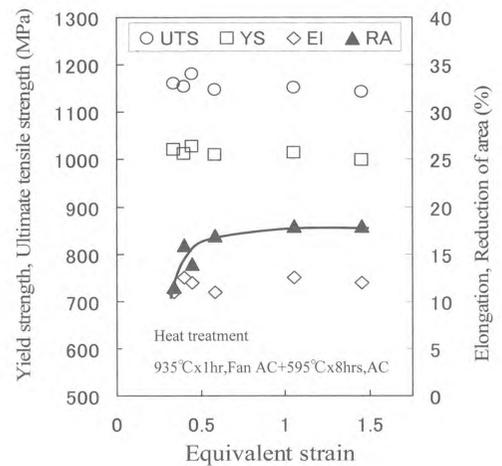
**Figure 4.** Influence of forging strain on tensile properties of Ti-6246  $\beta$ -processed forging (at RT)
