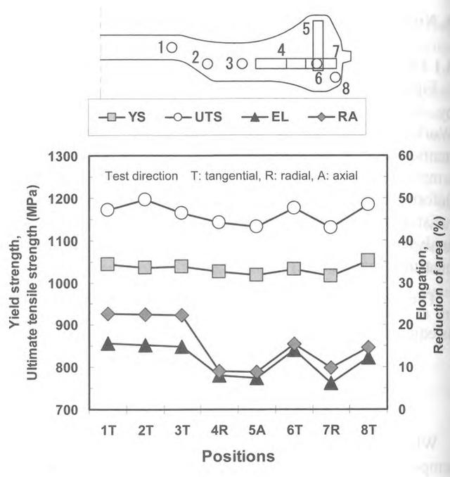
Figure 9. Results of tensile test of disc forging (at RT)
