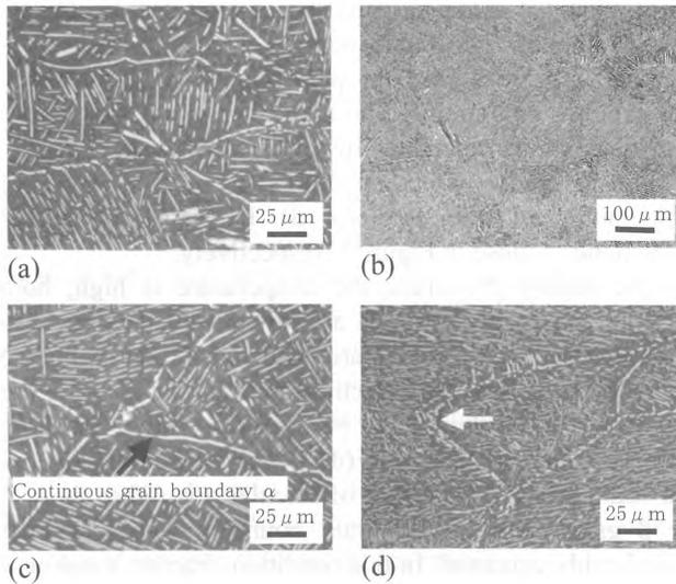
**Figure 3.** Microstructure of Ti-6246  $\beta$  processed forging
