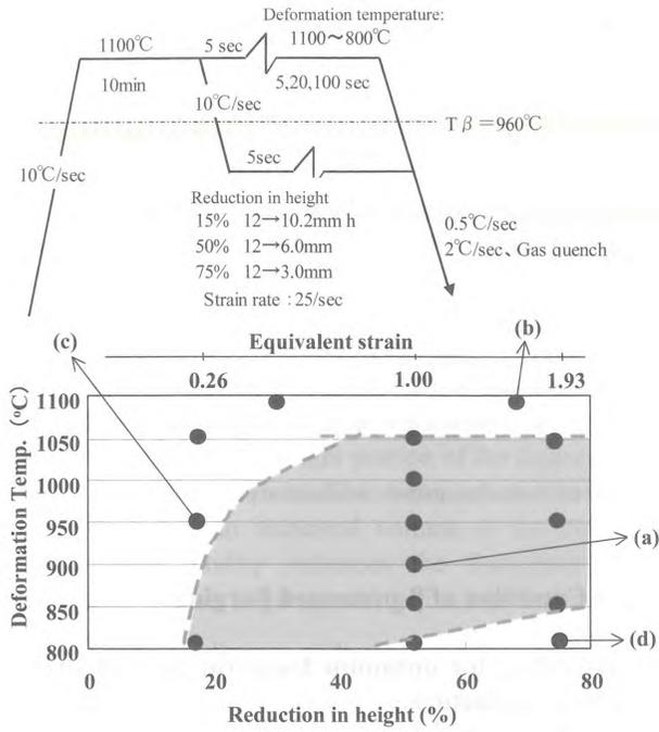
**Figure 2.** Influence of temperature and strain on microstructure of  $\beta$ -processed forging
