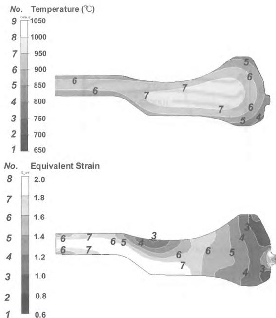
Figure 8. Results of calculation of temperature and strain during disc forging
