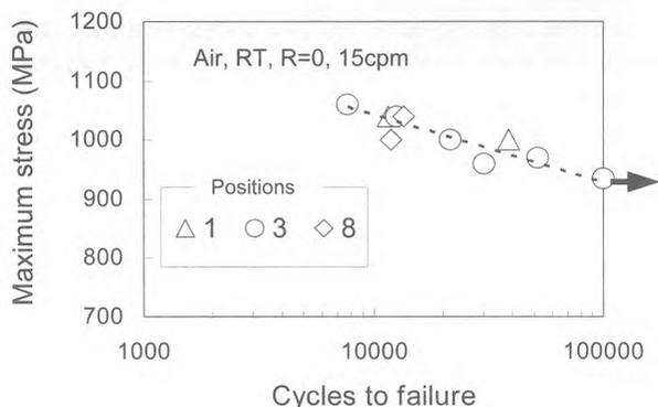
Figure 11. Results of LCF test of disc forging
