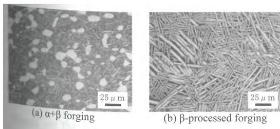
Figure 1. Microstructure of Ti-6246 forging
