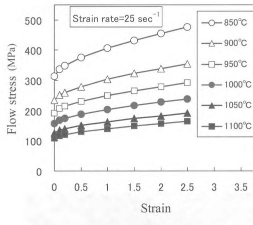
Figure 7. Isothermal flow stresses of Ti-6246
