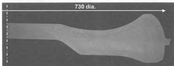
Figure 10. Macrostructure of beta-processed disc forging
