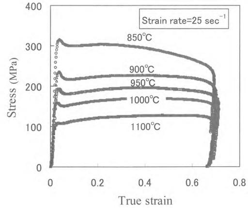
Figure 6. Stress-strain curves of Ti-6246
