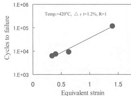
**Figure 5.** Influence of forging strain on LCF life of Ti-6246  $\beta$ -processed forging
