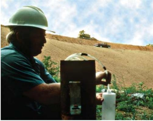
Testing of water samples in groundwater monitoring wells at modern landfills ensures that leachate collection systems are working correctly to protect public health and the environment.
