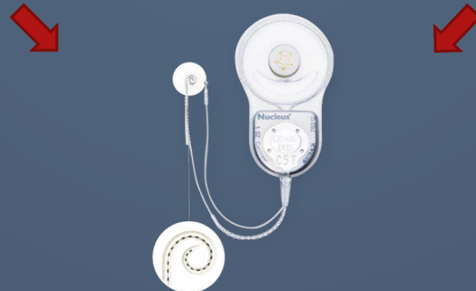
Cochlear Nucleus CI24RE CA / CI512 Contour Advance electrode array
