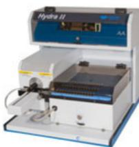
Teledyne Leeman Labs Hydra IIC is a fully automated turnkey analyzer that measures mercury in solid and semi-solid sample matrices directly without any acid digestion (sample preparation). The system employs the technique of sample combustion (thermal
