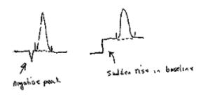
4.8 Properly integrated fused tailing peak (very difficult to accurately quantify). Do maintenance on chromatography system to avoid if possible).
