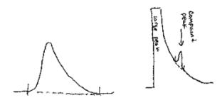
4.5 Properly integrated overload peak (i.e. benzoic acid on DB-5).
