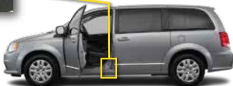
The **Tire Placard** label (required) is typically found on the driver side of the vehicle on what is called the “B” Pillar or may also be on the driver’s door edge. The load carrying capacity can be found on this label where it says “the combined weight of occupants and cargo shall never exceed.”
