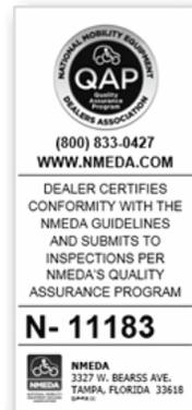
The **QAP** label (optional) is required to be placed on any vehicle modified with mobility equipment and sold by a NMEDA QAP dealer and is a certification from the dealer that the vehicle was modified in accordance with the QAP Rules and Guidelines and will have a unique serial number that is traceable to the dealer (or dealers if multiple QAP labels are applied) who performed the modification or who sold the vehicle.
