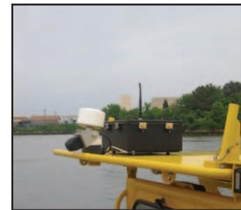
*Left to right: This high-tech security control terminal aboard the USV can be operated manually, or via remote control for many different types of missions. • A laptop computer is a key part of the USV terminal station. • An omnidirectional antenna and video cameras are perched atop the USV. • This Global Positioning System (GPS) antenna and receiver relay are key elements of the USV's control system.*
