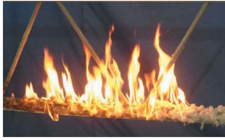
**Lint is extremely flammable. Once on fire, lint fires spread quickly. (Photo: courtesy of SonicAire®)**
