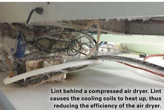
**Lint behind a compressed air dryer. Lint causes the cooling coils to heat up, thus reducing the efficiency of the air dryer.**
