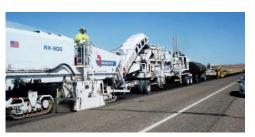
corrections may be made with a micro mill prior to application of the surface course. Using a micro mill for these corrections may eliminate shoving of the recycled layer compared to substitute methods such as diamond grinding. The nature of the smooth pattern and reduced contact pressures provided by the micro milling drum also minimizes impact to the recycled layer and prevents the unnecessary removal of excess recycled material.
