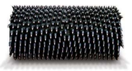
Since micro milling drums contain additional cutting teeth than a conventional milling drum, cutting depth in a micro milling application is limited. Micro milling is best utilized when the prescribed cutting depth is two inches or less. If rotomilling to a greater depth is necessary, the bulk of the existing material should first be removed with a conventional milling drum, then a micro milling drum may be utilized to remove the final one to two inches of material.
