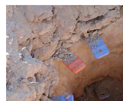
Figure 2. PRS probes in place on the Virgin River floodplain, in the soil profile.
