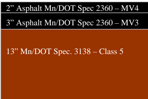
Austin Wal-Mart Typical Sections for "Heavy Duty" Pavement.
