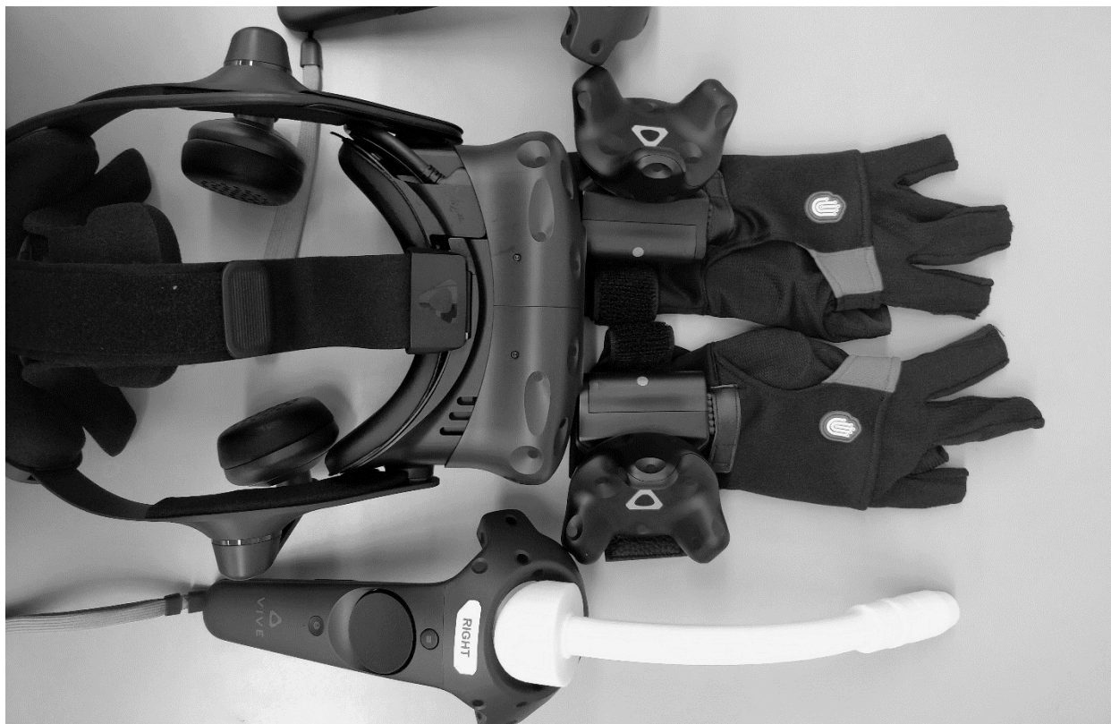
Figure 7. HTC Vive Pro and Noitom Hi5 VR glove along with 3D printed MIG Gun.
