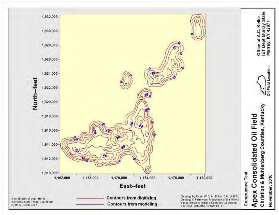
Figure 3 shows a typical contour validation map. If gridding and graphic contours were not congruent, supplemental contours or spot elevations were digitized on the legacy map. The process was repeated until the two sets of contours matched.
