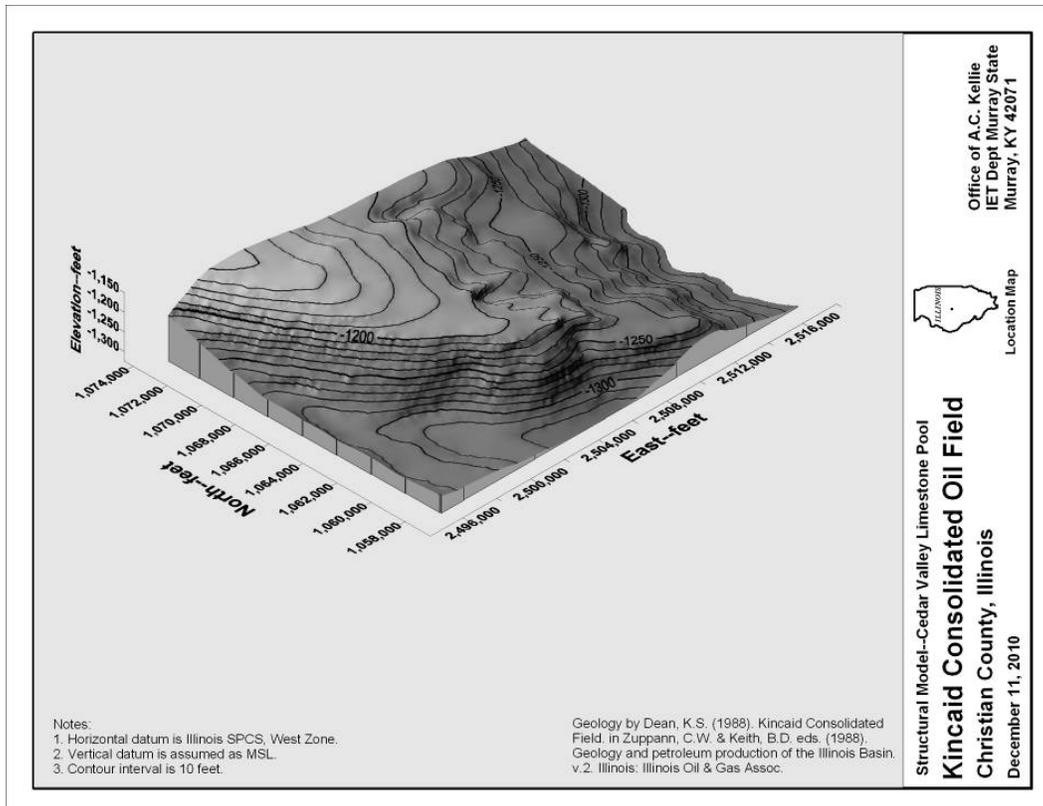
Contours are used to show surface elevation below sea level. An orthographic projection is employed with a model rotation of 45 degrees and a tilt of 35 degrees. The resulting view is from the southwest corner of the site.
