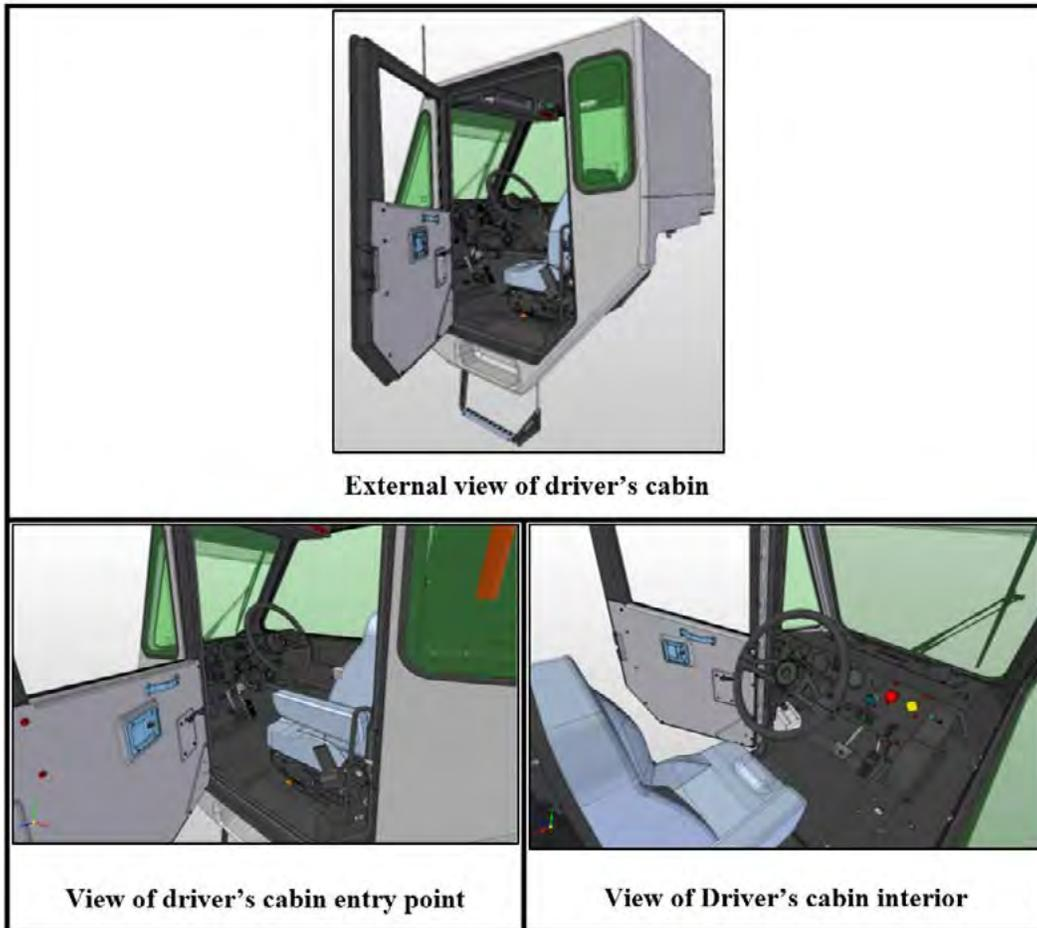
**Figure 5. Developed CAD model of driver's cabin**
