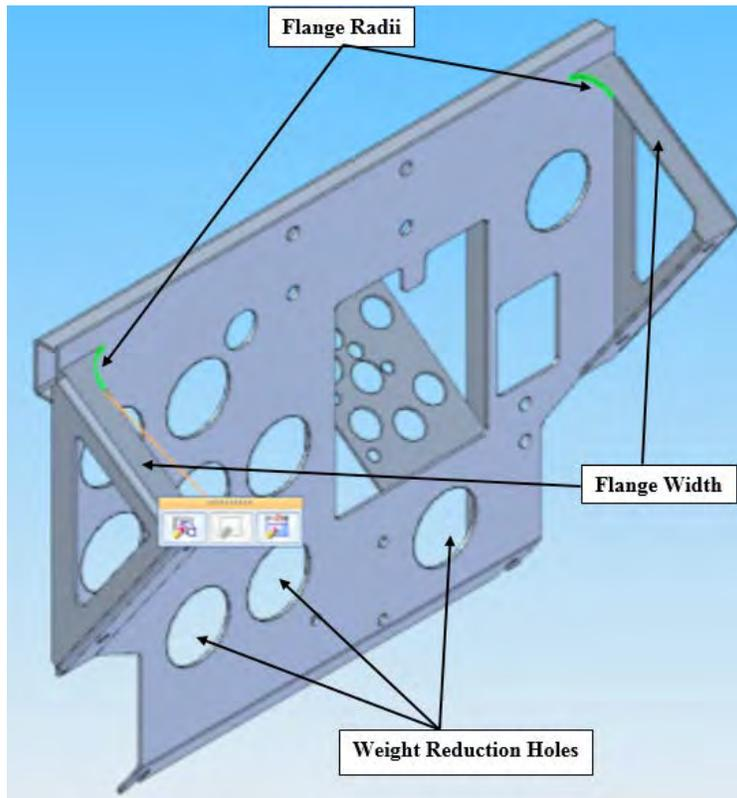
**Figure 3. Three design features (factors) within the mounting bracket**
