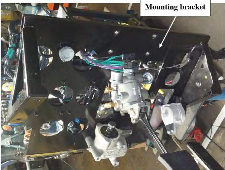
**Figure 2. Actual steering column bracket sub-assembly**
