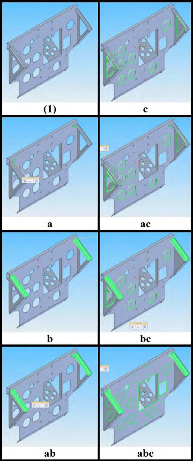
Figure 7. CAD models for 8 unique design alternatives of the mounting bracket
