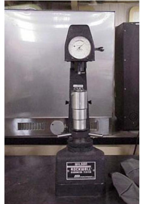
**Figure 3. Rockwell Hardness Tester**
