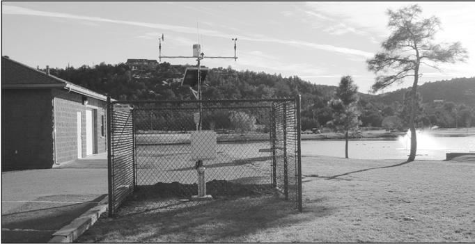
*This weather station in Green Valley Park provides information that can be used for drought mitigation and water conservation efforts. Currently, the station monitors for precipitation, wind speed, solar radiation, relative humidity, and air and soil temperature. Evapotranspiration rates are calculated for more accurate outdoor irrigation.*
