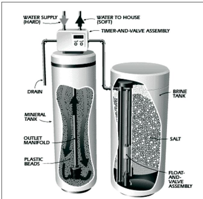
That solution is used to flush the resin tank, forcing the calcium and magnesium ions off the resin bead and replacing them with sodium. A meter at the top of the resin tank regulates these flush (regeneration) cycles. It is set based upon the hardness value for the water – one grain-per-gallon equals 17.1 mg/l total hardness. Phoenix area water ranges between 17 and 22 grains of hardness.
